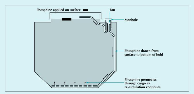
Fumigation of cargo in ship's hold using phosphine and a powered re-circulation system
