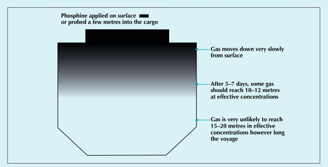
Traditional fumigation of cargo in ship's hold using phosphine
